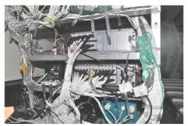
stalled in the aircraft and the sensors are attached to a customer-specific connector panel equipped with the desired connector types.
