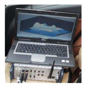
Volkswagen's acoustic analysis system is used throughout the world and in conjunction with imc CRONOS-PL VMS direct, time-saving, and economical analysis of the acoustic impact on a car interior.
